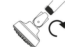
2 Hand tighten Evolve Handshower Mount clockwise onto the shower pipe.
